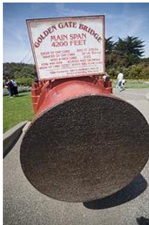
The weight of the roadway is hung from two cables that pass through the two main towers and are fixed in concrete at each end. Each cable is made of 27,572 strands of wire. There are 80,000 miles (130,000 km) of wire in the main cables.
